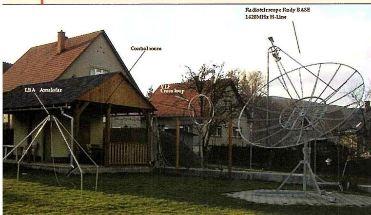
Obr. 1. Rádioteleskop BASE (Bojnice Amateur Space Ear).
